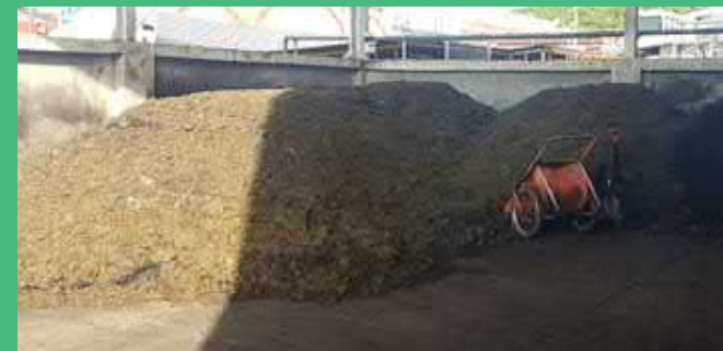
62 The tea leaves used in the production of C2 ready-to-drink beverage are collected and used as alternative fuel for boiler.
